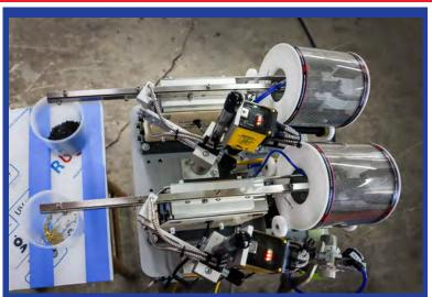
As the drum rotates, the ribs inside the drum agitate and orient your parts, transporting the parts to the liner track or belting system.
