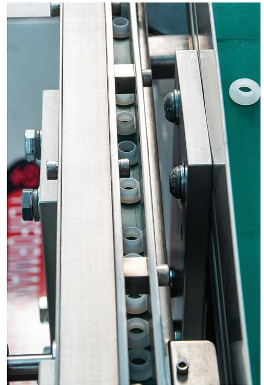
Correctly oriented parts exiting the step feeder.
