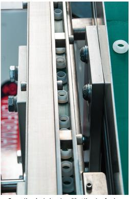
Correctly oriented parts exiting the step feeder.
