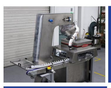
The Performance Feeders Bottle Unscrambler with Slant Disc Feeders function is to feed a bulk supply of containers and orient them for packaging processes. The Performance Feeders Bottle Unscrambler is designed to feed a variety of containers with 100% orientation at varying speeds of 5 parts per minute to 200 parts per minute, using minimal floorspace.
