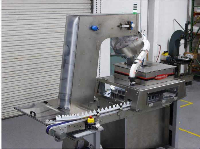
The Performance Feeders Bottle Unscrambler with Slant Disc Feeders function is to feed a bulk supply of containers and orient them for packaging processes. The Performance Feeders Bottle Unscrambler is designed to feed a variety of containers with 100% orientation at varying speeds of 5 parts per minute to 200 parts per minute, using minimal floorspace.
