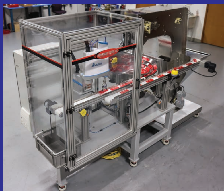
Vibratory Conical Feeder with Delta SCARA Robot
